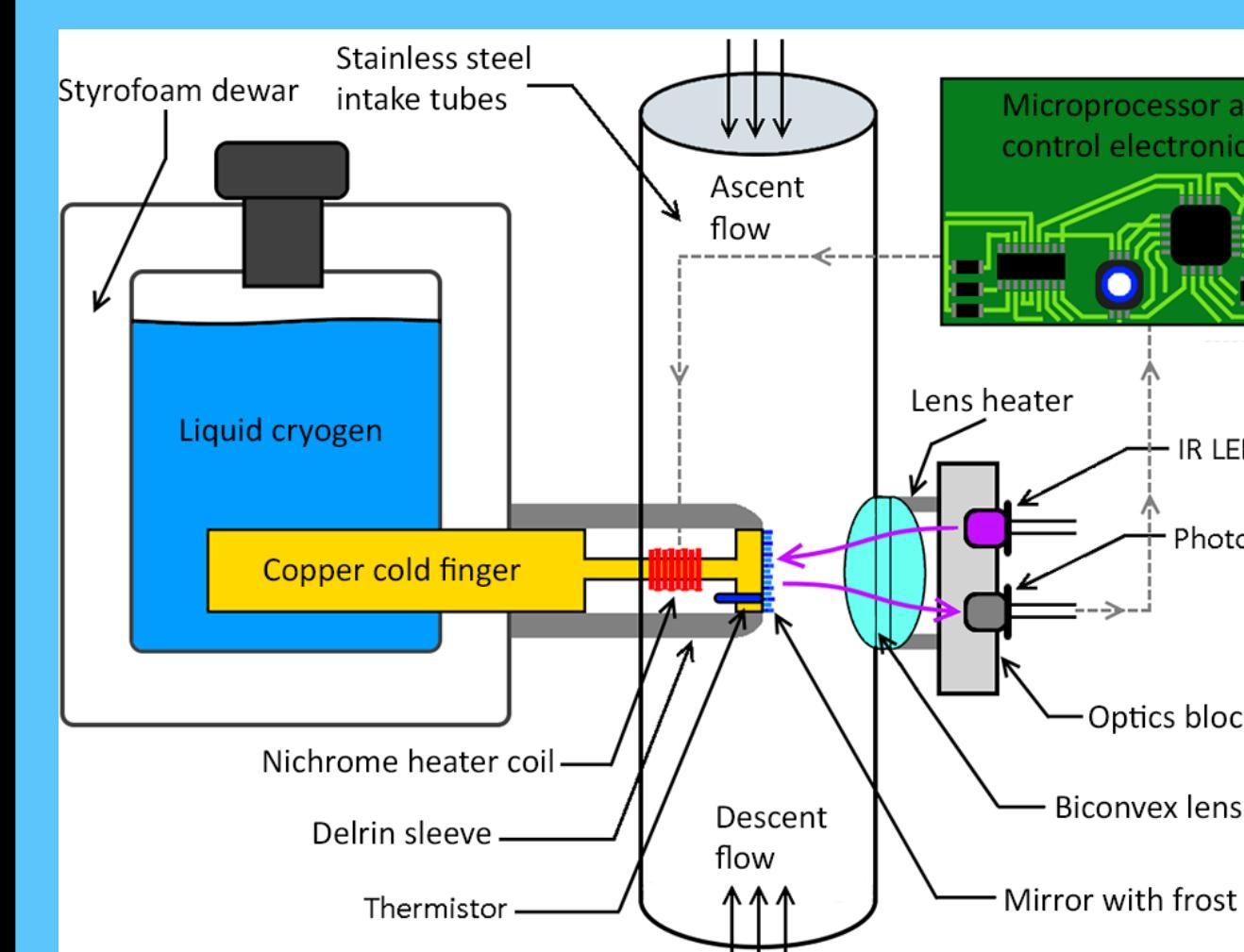
The NOAA FPH relies on maintaining a thin, stable layer of condensate on a mirror through rapid feedback control. A calibrated thermistor embedded in the mirror accurately measures the frost point temperature. The Goff-Gratch formulation of the Clausius-Clapeyron equation is used to calculate the water vapor partial pressure.
