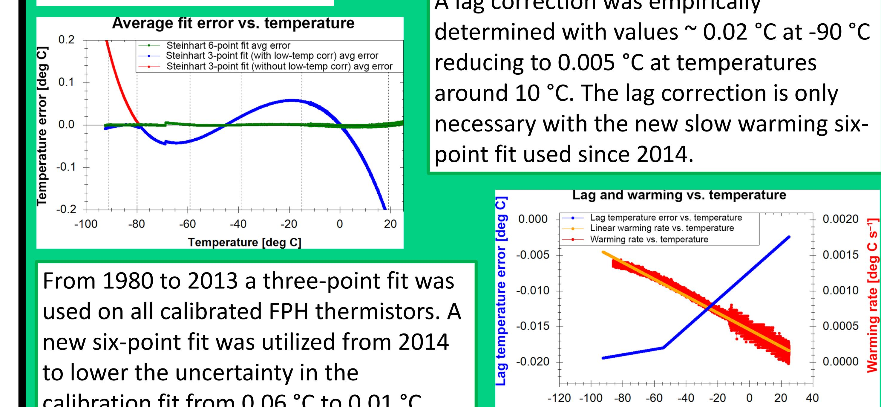
From 1980 to 2013 a three-point fit was used on all calibrated FPH thermistors. A new six-point fit was utilized from 2014 to lower the uncertainty in the calibration fit from 0.06 °C to 0.01 °C.
