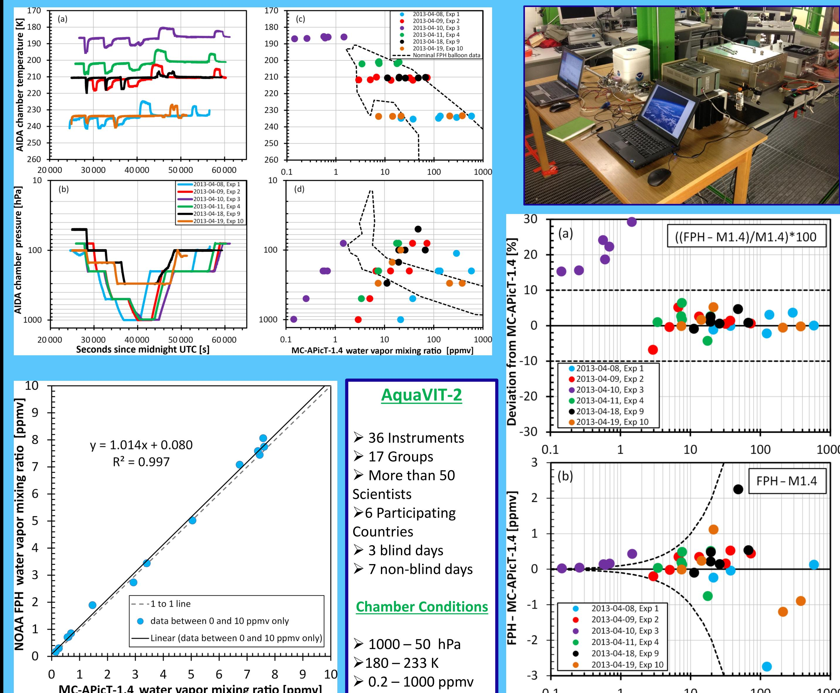
A total of 36 stable sections were analyzed lasting roughly 30 minutes each in duration. The NOAA FPH agrees with the MC-APicT-14 instrument within 10% between 2 and 600 ppmv. Below 1.5 ppmv the agreement is better than 30%.
