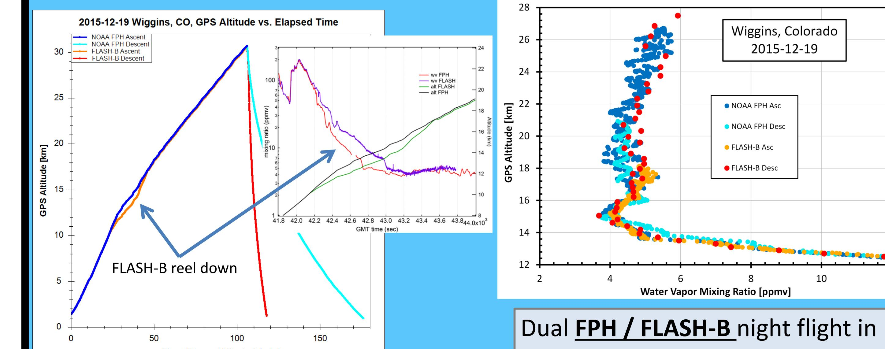
FLASH-B was reeled down 1000 m below the FPH at 10 km. It was reeled back in by 17 km but the package was stuck 130 m below the FPH due to a small reel issue.
